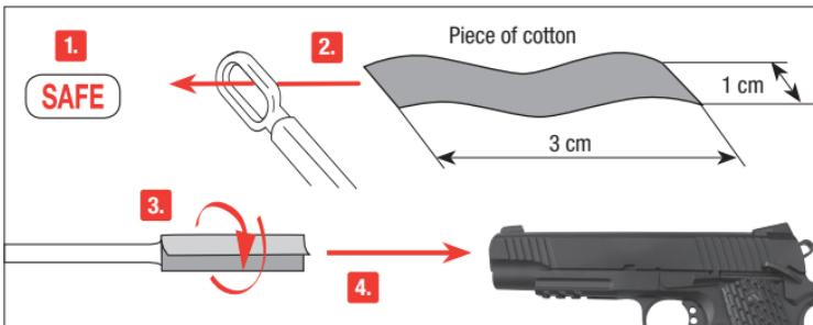
Put the safety on "safe". Prepare a thin rod with a length of approx. 10 cm. Attach a piece of cotton fabric to its end and clean the barrel with some silicone oil.
