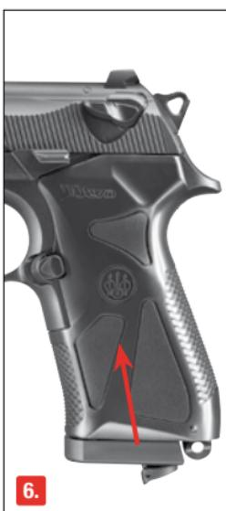
The magazine can be removed only when the hammer is decocked. Press magazine release. Remove the magazine.
