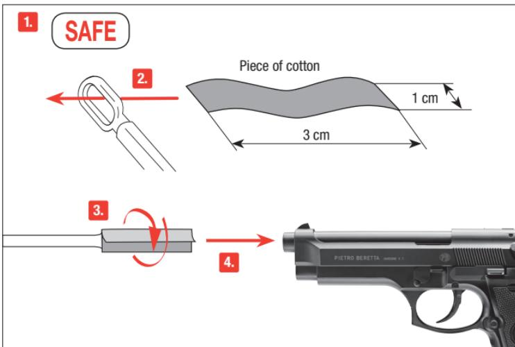
Put the safety on "safe". Prepare a thin rod with a length of approx. 30 cm. Attach a piece of cotton fabric to its end and clean the barrel with some silicone oil.
