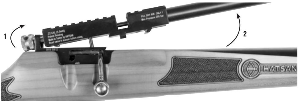
Take the other barrel/mechanism of different caliber in your hand and insert it on the air rifle as shown **(Fig13)**. While doing this make sure the you align the pin into the its hole in the air rifle body.
