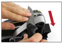
Continue sharpening the same side of the blade until a burr is raised along entire edge (count strokes).
