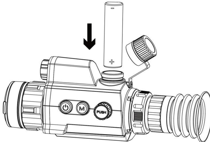
Figure 2-3 Install Battery
