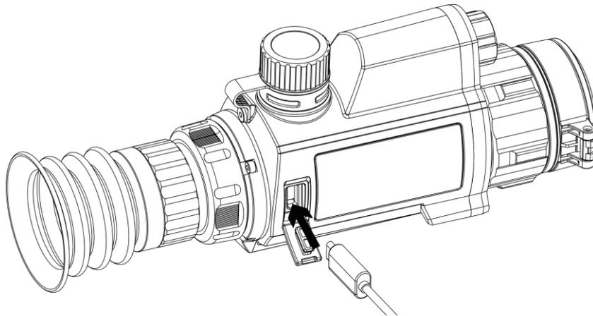
Figure 2-1 Cable Connection
