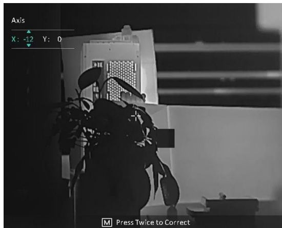
Figure 3-6 Correct Defective Pixel
