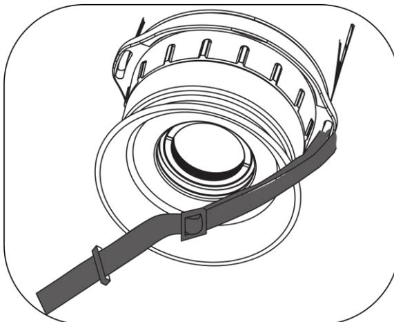
Figure 2-8 Thread Neck Strap through Strap Keeper
