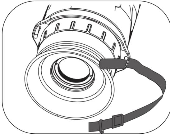
Figure 2-6 Thread Neck Strap through Attachment Point
