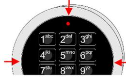
1. Remove the keypad from its bracket by carefully lifting the keypad with a flat, blunt screwdriver placed under the edge of the panel between keys 4 and 7, between keys 6 and 9, and above the LED (see illustration).
