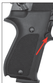
Press the grip plate release button.
