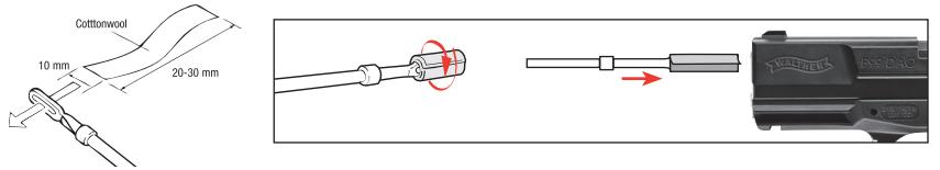
Put the safety on „safe“, remove the magazine. Prepare a thin rod with a length of 30 cm.
