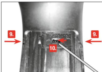
9. Insert the magazine catch while holding up the counter support.
