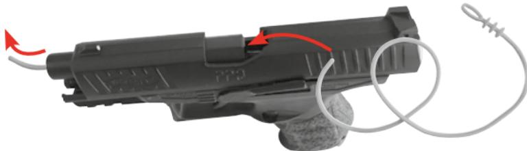
Pull back the slide and hold it. Pull the squeezy through the barrel to clean it.
