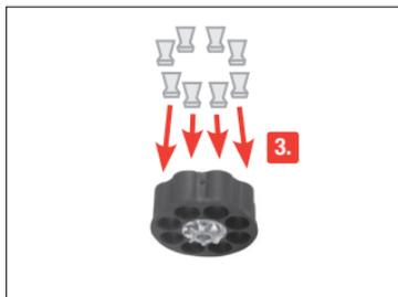
3. Load pellets. Ring gear points down.
