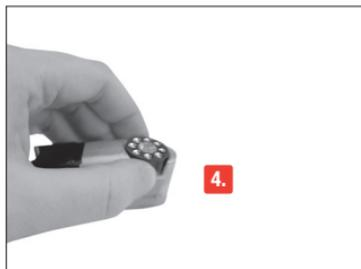
4. Insert cylinder rotary clip in loading position. Ring gear points up.
