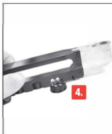
4. Press magazine onto rotary clip. Ring gear points down.
