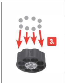
3. Load Steel BBs. Ring gear points down.
