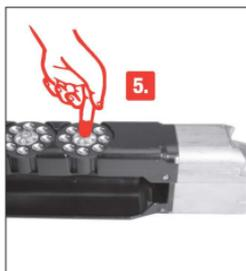
5. Press rotary clip firmly into place. Ring gear points up.
