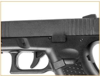
Pic. 1 b) Side fuse, unlocked.
